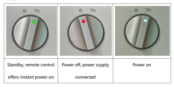
Power On: After the power is connected, turn the front power knob to the ON position. The indicator will turn white, the display will light up, and the K17 will power on.
