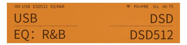
Mode Selection Interface: Swipe left to switch between 8 working modes (USB, Optical, Bluetooth, Streaming, Coaxial, Line Input, Balanced Input, Local Playback).
