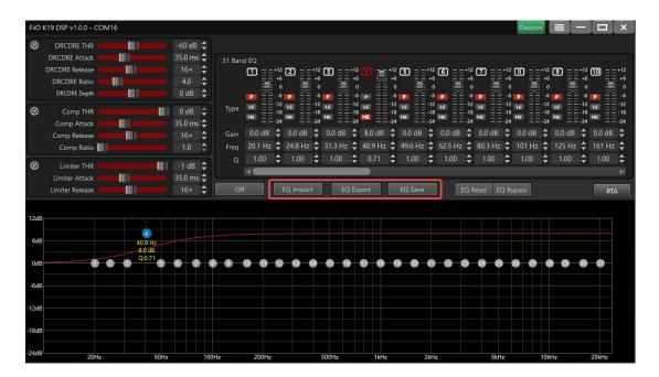
When you click "EQ Export" the current EQ settings can be saved to your computer as a local parameter file with an .XML extension. Clicking "Import EQ" allows you to load an EQ parameter file into the DSP client, and the K19/K1 will immediately apply the settings. Exporting files makes it easy to share with others. FiiO also provides tuning curves for some headphones—contact customer service for details.
