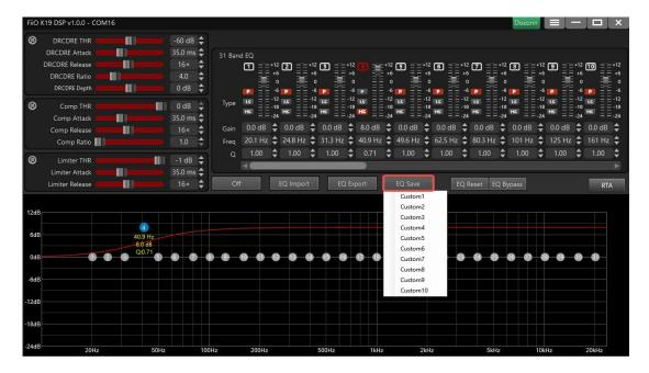
When the DSP client is connected, any imported or modified EQ settings will take effect immediately on the K19/K17. However, the changes will not be st ored permanently. To save the parameters to the K19/K17, click the "Save EQ" button and store them in Custom 1–Custom 10, overwriting the previous cu stom settings.
