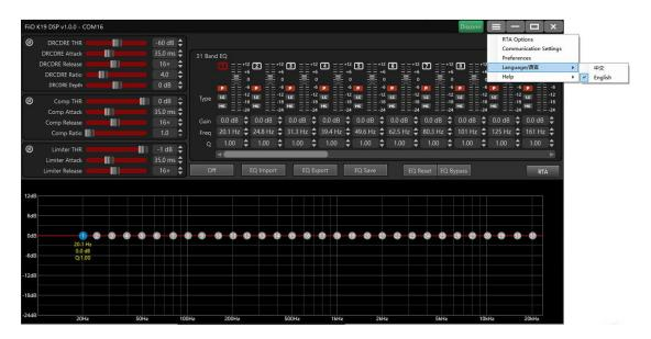
As shown in the figure below, you can select the PEQ settings. When "Custo m" is selected, you can adjust the curve interface at the bottom to set your preferred curve. After setting the curve, you need to click "Save EQ" and cho ose a save location to store the curve on the K17 device.
